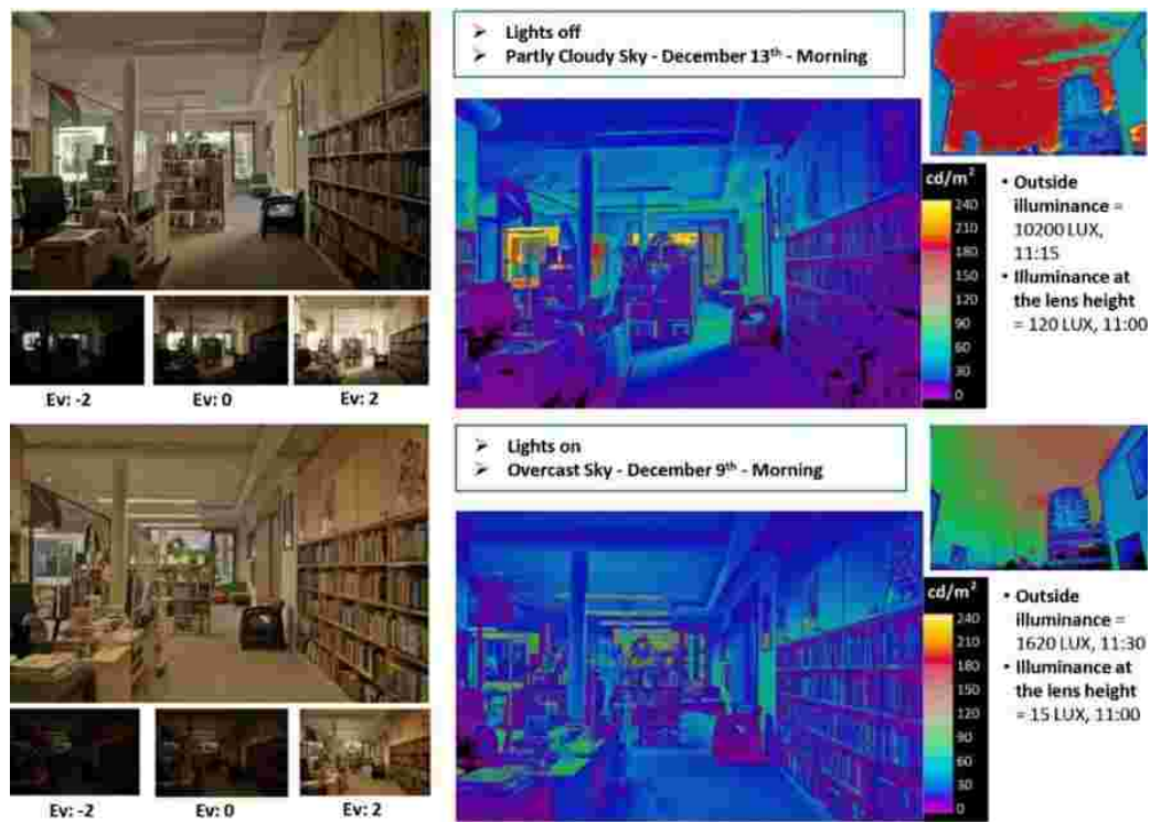
Figure 3.4. False color images showing the luminance difference in the Witomino (first floor) (source: author).
