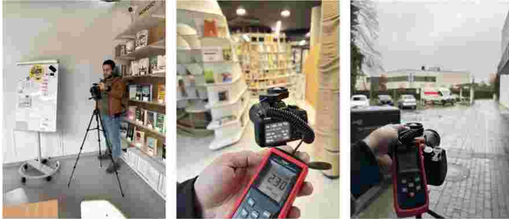
Figure 3.1. The setting for the HDR photography included readings of the illuminance level at the height of the camera lens (Pictures by author).
