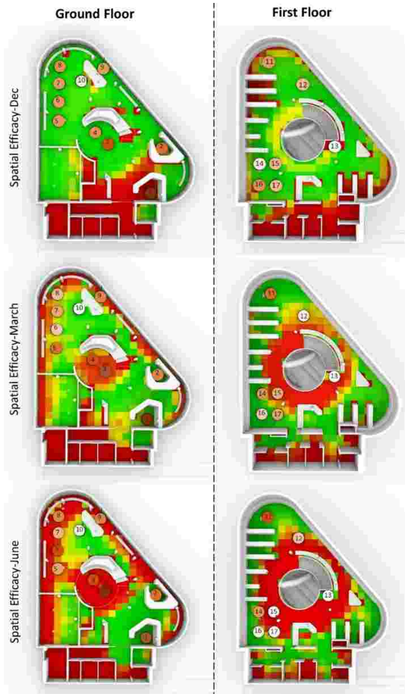
Figure 4.20. Spatial efficacy overlaid on UDI simulation results for the Maly Kack Library.
